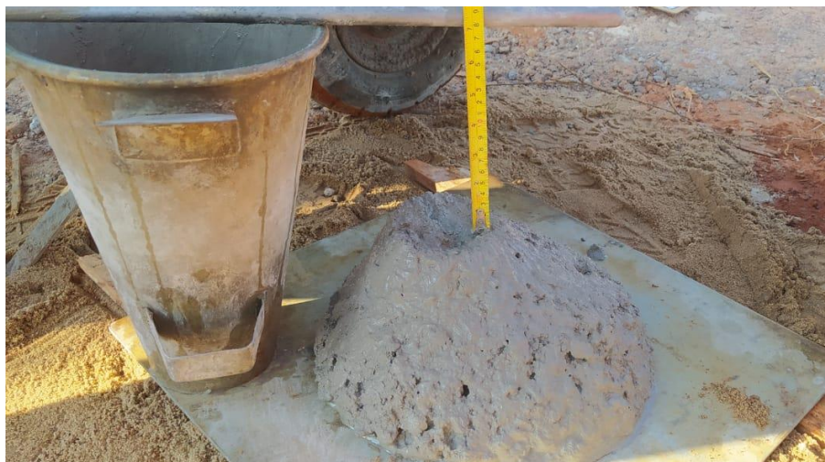
Figura 48 – Slump test reprovado
