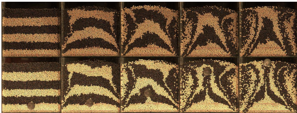
Figure 14 – Evolution of the vibrated bed. Top Panels are without intruder, while bottom Panels are with an intruder. Black and yellow layers are made of mustard grains. Figure taken from [64].
